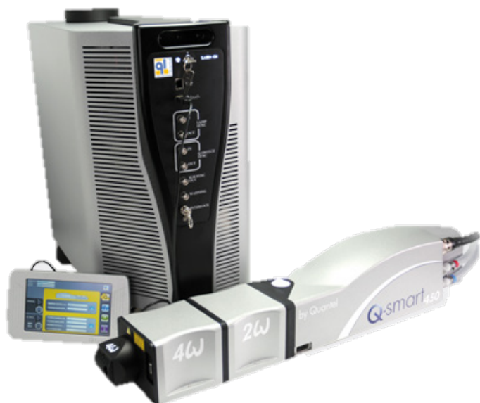
Figure 1. High power 450 mJ/p laser equipment for the production of AuNPs by laser ablation.
