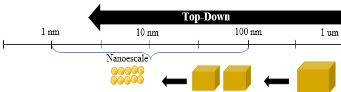
Figure 2. Top-down approach to gold nanoparticle production.
