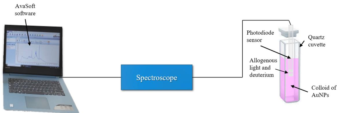
Figure 3. Characterization diagram of AuNPs in colloidal state.
