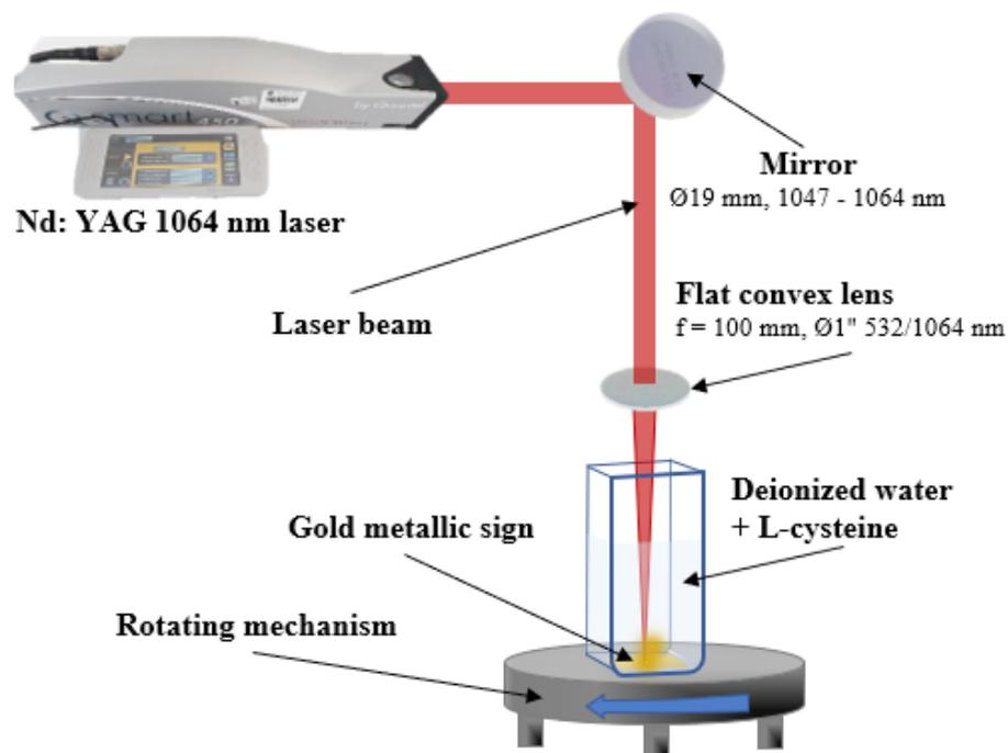
Figure 4. Functionalization of gold nanoparticles with L-cysteine.
